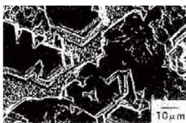
Fig. 2 Surface morphology of Zinc film electroplated on Cu single crystals <sup>[2]</sup>
